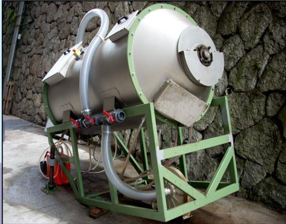
Dynamic Composting Reactor of 1500 L.
