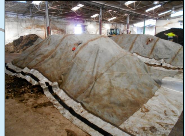
Pilot Plant of Windrow aerated piles w/ semi-permeable cover
